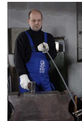
Setting the Shape of Blade
